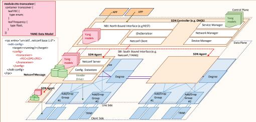
Fig.3. SDN Control of a disaggregated optical network (transceiver and/or optical line system)
