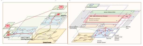
Fig. 1. (a) Metro-Haul Infrastructure, showing the main components: the disaggregated transport network interconnecting Metro-Haul locations (AMEN/MCEN nodes), the packet switched networks and the NFVI PoP encompassing computing, storage resources. (b) Macroscopic view of the Metro-Haul Control, Orchestration and Management (COM) and Service Platform, highlighting the NFV MANO part, the hierarchical SDN control, the Monitoring and data analytics (MDA) and Network Planning (NP) components
