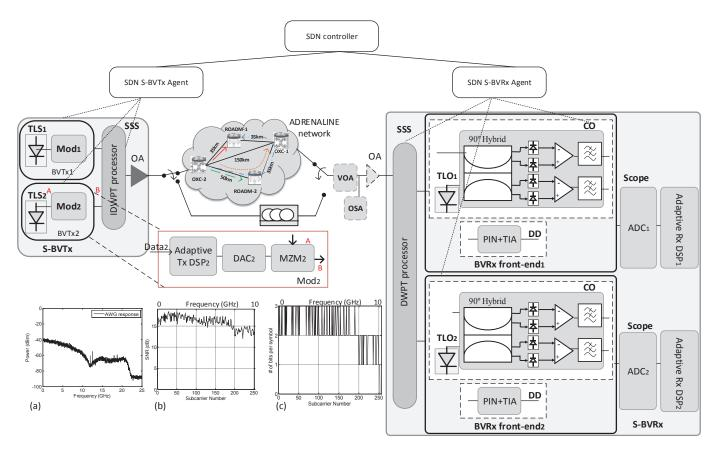
Fig. 4. Experimental set-up for the proof of concept. In the inset of the figure, (a) AWG transfer function and example of (b) estimated SNR and (c) bit assignment per subcarrier considering AM and CO reception
