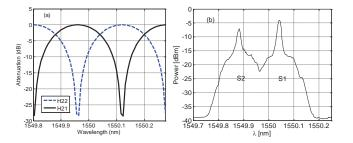
Fig. 3. (a) MZI transfer function emulating the Haar wavelet and considering 40 GHz FSR (b) OSA capture of the two multiplexed slices with a 0.4 nm resolution bandwidth
