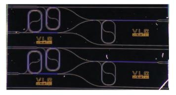
Fig. 2. PIC-based IDWPT/DWPT optical orthogonal transform processors corresponding to a 2-levels decomposition Haar wavelet
