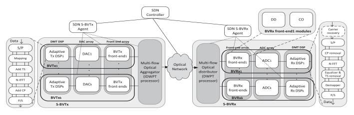
Fig. 1. Programmable SDN-enabled S-BVT architecture
