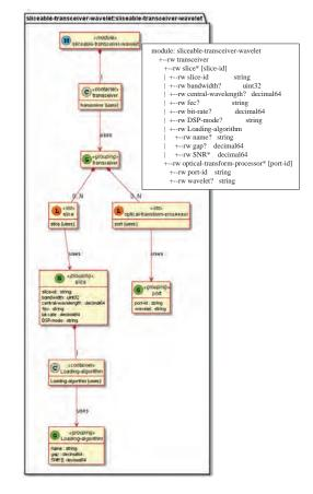
Fig. 6. S-BVT YANG model in UML
