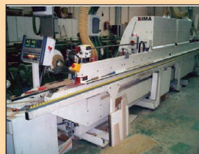
CANTEADORA IMA ADVANTAGE EXPERT/6216/L 12 Espesor: canto 12 mm. / material 3 mm.
