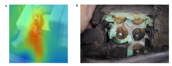
Fig. 2 (a) Thermal image of the positive terminal of a car battery which indicates a poor connection, marker displays degrees Celsius; (b) Oxides in a terminal block detected by a thermal imaging camera
