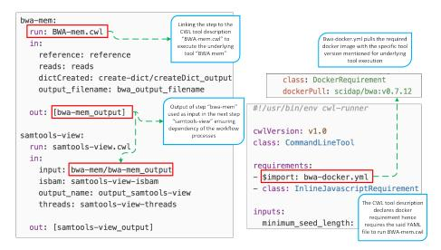
Figure 2. Right: A snapshot of part of a GATK workflow described using CWL. Two steps named as *bwa-mem* and *samtools-view* are shown where the former links to the tool description executing the underlying tool (BWA-mem for alignment) and provides the output used as input for samtools. Left: Snapshot of BWA-mem.cwl and the associated Docker requirements for the exact tool version used in the workflow execution.
