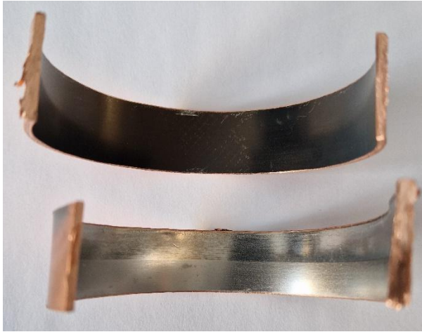
Figure 3. Photos of nonirradiated surface (upper image) and irradiated by Nb:YAG laser of tubular part of inner surface of RF cavity (under image). After laser irradiation, the roughness parameters R_a decreased by about an order of magnitude from 900 nm to 90 nm.
