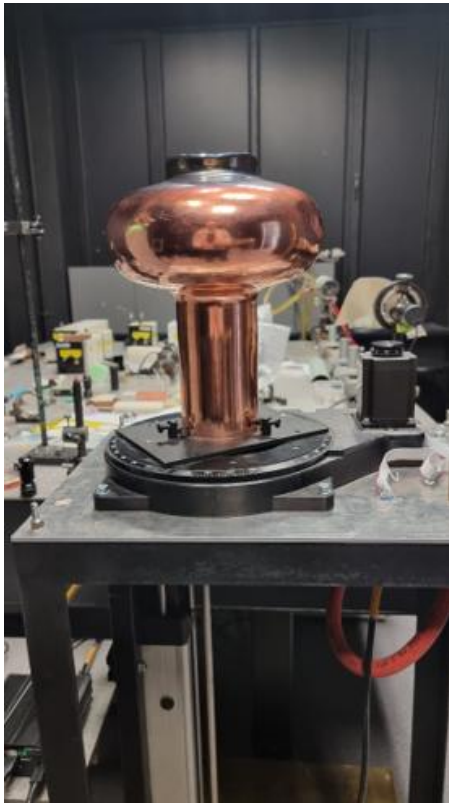
Figure 4. Photo of construction of Ar gas chamber with controlling 3D coordinates for laser treatment of the RF 1.3 GHz cavity with Nb thin film in the inner surface.
