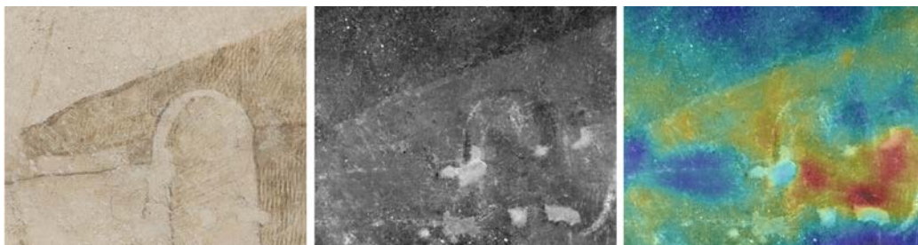
Figure 10: Example of dual-mode imaging for diagnostics in a fresco detail: visible (left); TQR measurement (center); alpha fusion image between TQR and thermogram after the lamps switch-off (right).
