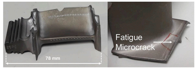
Fig. 1. Inconel aircraft engine turbine blade with a 1.4 mm fatigue micro-crack in its shroud.
