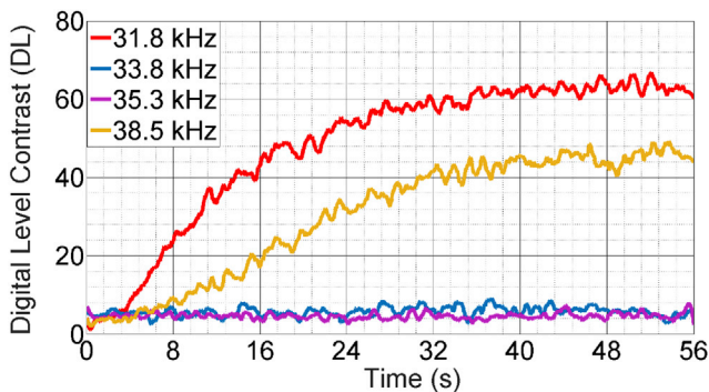
Fig. 11. Comparison of NACT thermal amplitude contrast variation for the four investigated driving frequencies, i.e. 31.8 kHz, 33.8 kHz, 35.3 kHz and 38.5 kHz.
