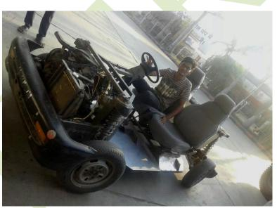
Fabrication model of four wheel steering system of Maruti 800.
