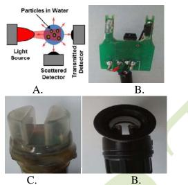
Fig.2 Turbidity sensor. (A) Measurement principle. (B) Probe board. (C) Flat surface PTFE housing. (D) Inline Tee fitting
