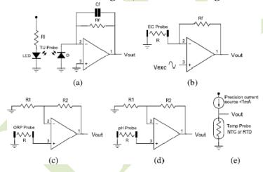
Fig. 3. The first stage of analog signal conditioning circuitry. (a) Turbidity preamplifier. (b) Conductivity preamplifier. (c) ORP preamplifier. (d) pH preamplifier. (e) Temp.
