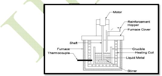
Fig 1 Schematic view of stir casting setup
