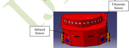
Figure 4: Front view of the Robot.
