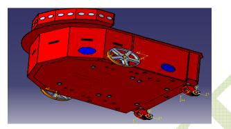
Figure 3: Wheel configuration of the Robot.
