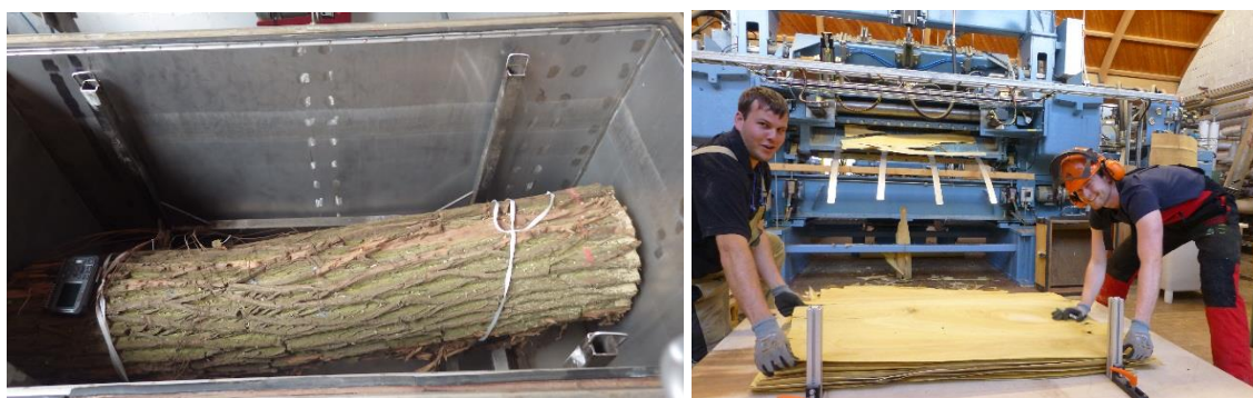
Figure 1: A Robinia log in the cooking unit (left) and the new RAUTE peeling machine at the WKI (right)
