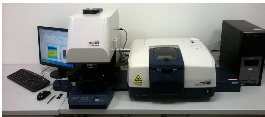
Figure 1: JASCO IRT-5000 infra-red microscope and JASCO FT/IR-6300 spectrometer (University of Sopron)
