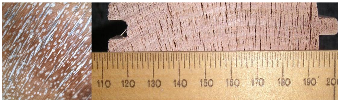
Figure 1. Blue gum wood cross cut (left) after Moderate degree MW modification. Narrow white lines are original rays, wider white lines are ruptured rays. Mountain Ash (right) wood structure after High degree MW modification.
