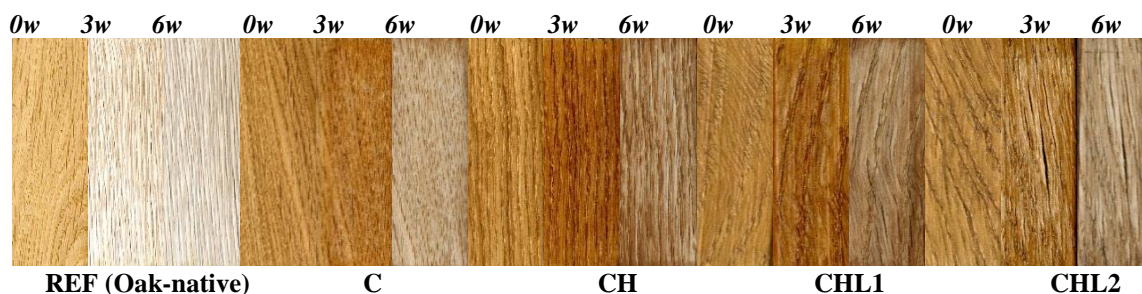
Figure 3: Visual changes of oak wood with different coatings during 6 weeks of accelerated weathering
