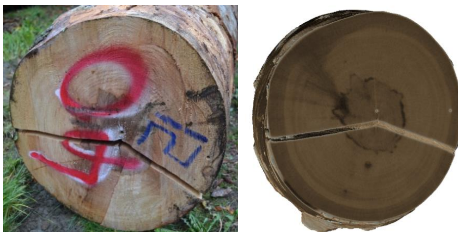
Figure 3: Comparison of wood characteristics within a beech log (left: photo, right: CT-image) ©MiCROTEC
