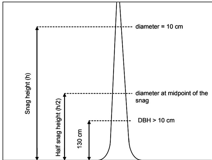
Figure 4. Procedure for snag diameter and snag height measurement.
