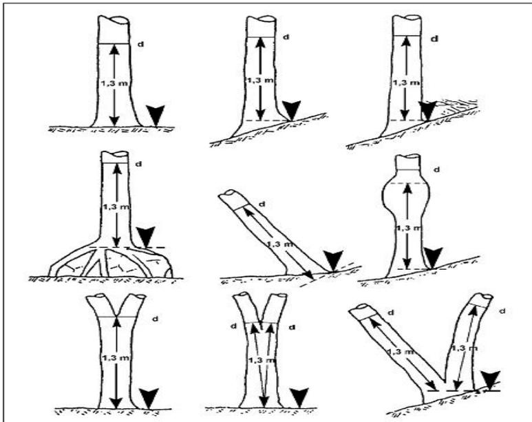
Figure 2. Guidelines for the measurements of DBH (diameter at 130 cm) in special cases.
