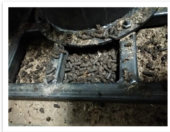
Fig: 5. Quantity of Pellets formed in one run of the machine
