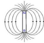
Magnetic fields are invisible fields that exert a vector force, characterized by both strength and direction, and are produced by changing electric fields (or magnetic objects).
