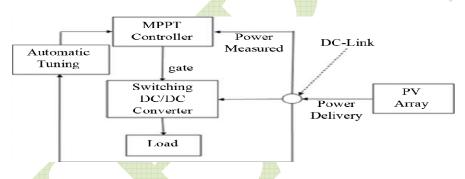
Fig. 4. Block diagram of adaptive Hill-climbing technique [7]
