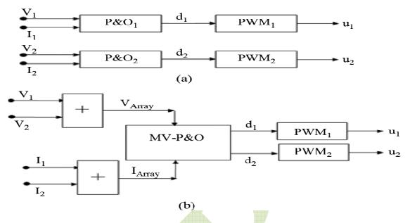
Fig.8. Comparison between (a) traditional P&O and (b) multivariable P&O Structures [7]
