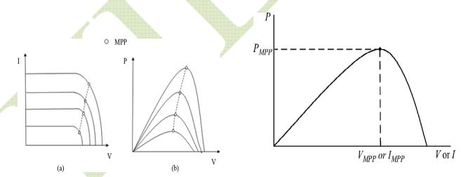
Fig. 1. (a) I–V and (b) P –V characteristics of PV panel at different environmental conditions.[7]
