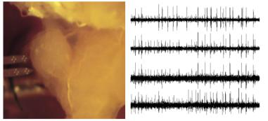
Left, the brain of an insect with the recording probe on which 16 electrodes (the bright spots) have been etched. Each probe's branch has a 80  $\mu m$  width. Right, 1 sec of data from 4 electrodes. The spikes are the action potentials.
