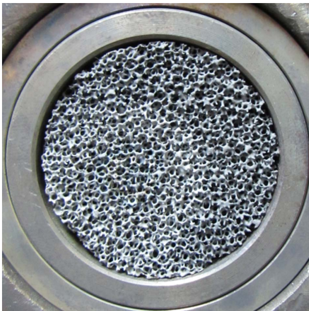
Fig. 17. Close view of the absorber sample placed in the receiver tube (Case I according to Table 1).
