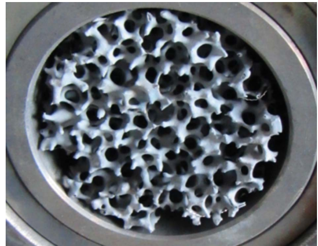
Fig. 1. Ceramic foam absorber sample placed in solar simulator test bed.
