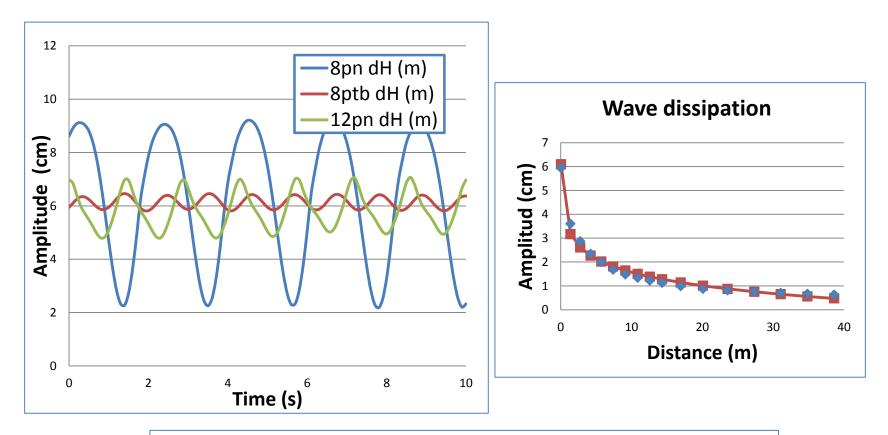
Amplitude of the waves generated by different paddle-wheels
