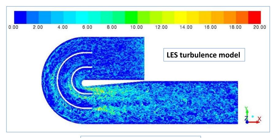
Isocontours of turbulent viscosity
