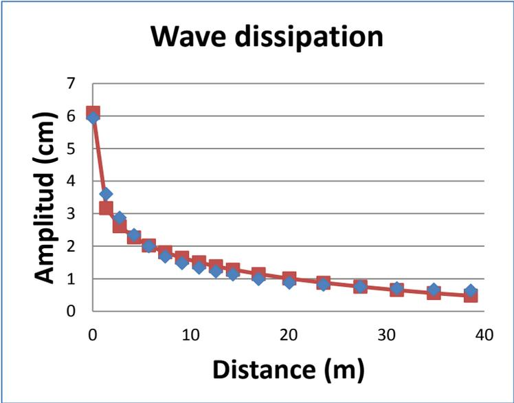
Amplitude of the waves generated by different paddle-wheels
