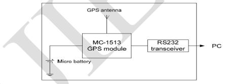
Fig.5 . Block diagram of GPS LS20032
