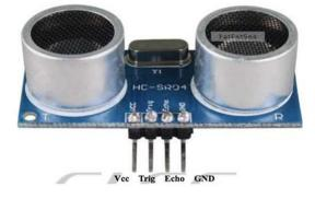
Fig.4. Ultrasonic Sensor
