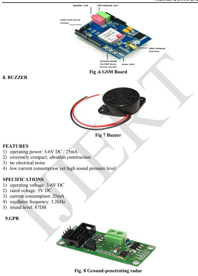
Ground-penetrating radar (GPR) is a geophysical method. It will uses radar pulses to image the subsurface. This nondestructive method uses electromagnetic radiation in the microwave band such as UHF/VHF
