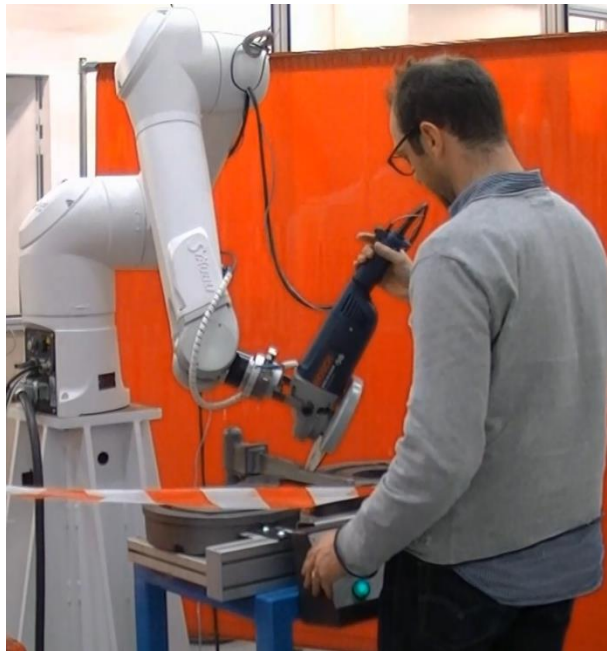
Figure 20: Learning by demonstration testing for OPSA in CEA CC
