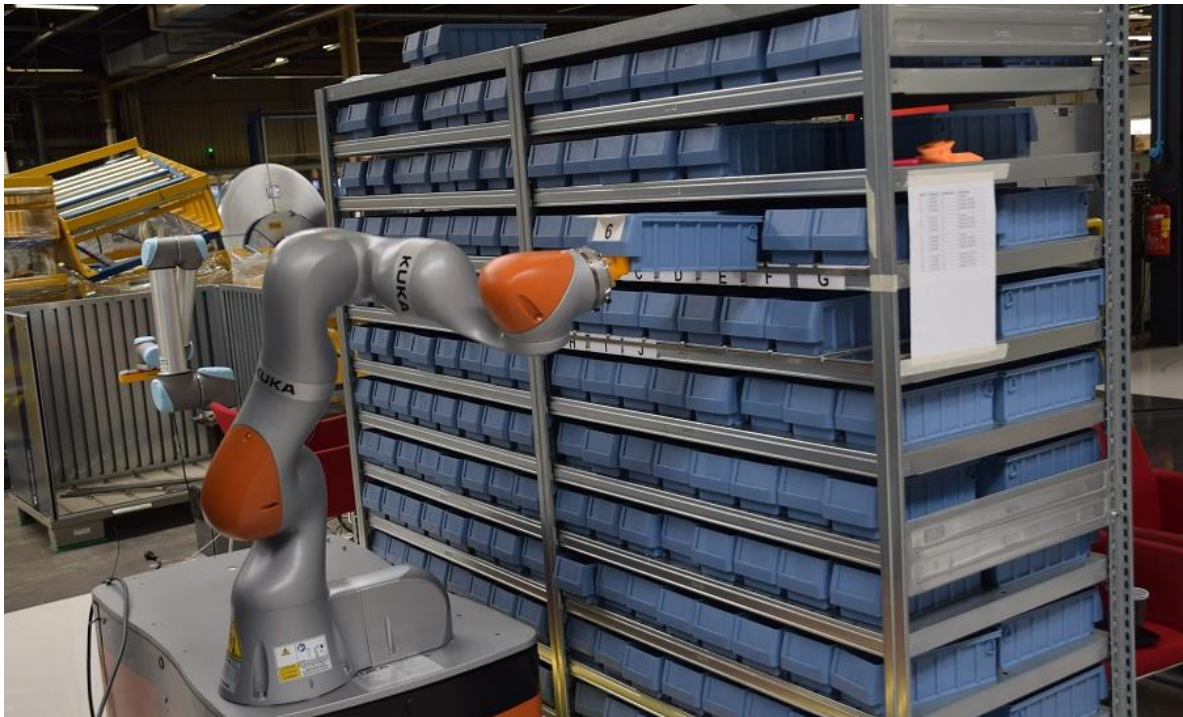
Figure 28: Mobile robot picks up tooling box for TRI P1 (at the background: UR robot of P1 loading)
