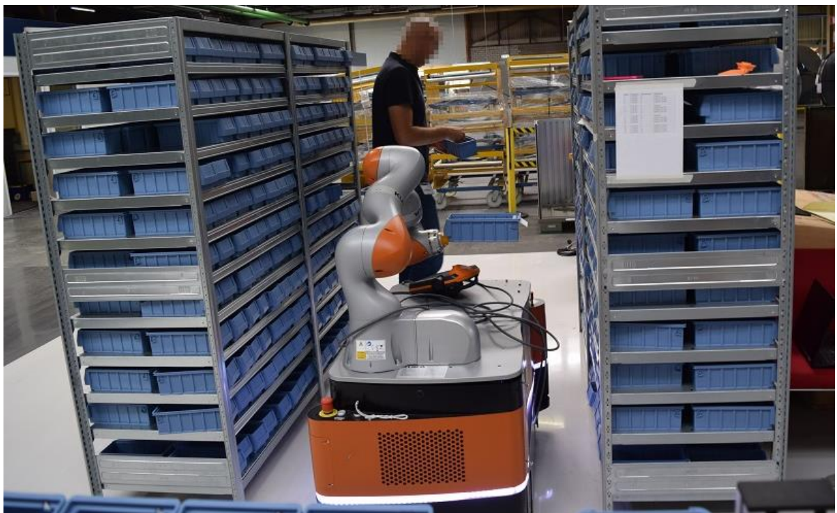
Figure 31: Mobile robot and worker in the same workspace (TRI P1)
