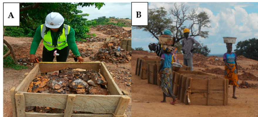
Figure 8. Evaluation of barite production in Azara, Nasarawa State, Nigeria using wooden boxes (A) researcher measuring the quantity unit box with (0.9 \times 0.9 \times 0.6) m, (B) respondents filling the boxes. Photo credit-authors.
