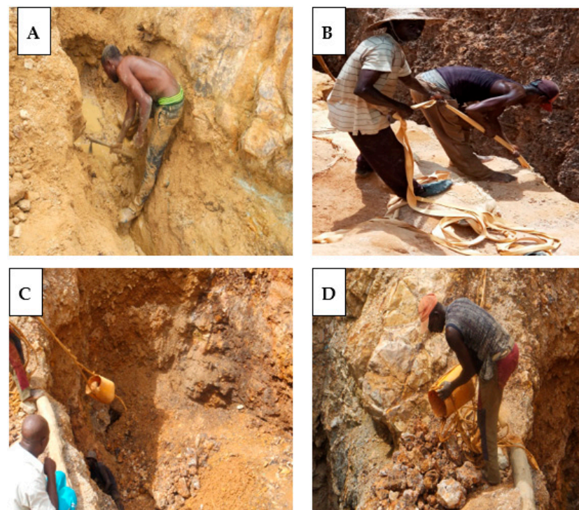
Figure 7. Mining and other activities using crude implements (A) excavating using crude implements such as hoe; (B–D) excavated minerals are carried from the pit to the earth surface using plastic bucket and rope.
