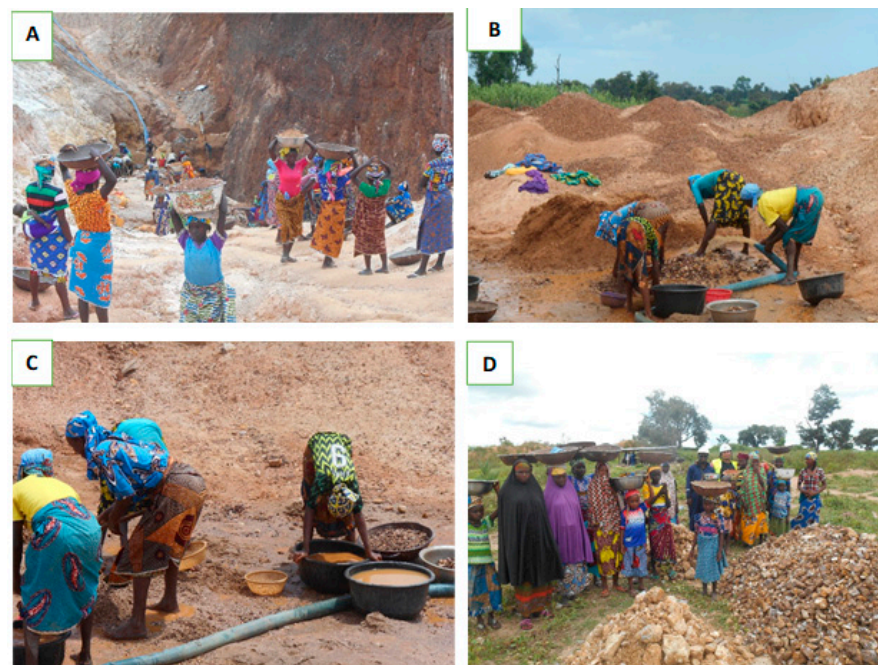
Figure 9. Women involvement in barite production in Azara, Nasarawa state (A) women transferring run-of-mine ore to designated washing point; (B,C) washing of barite by women; (D) stacking of barite at collection area. Photo credit: authors.
