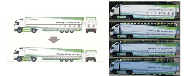
Fig. 4 Energy Efficiency or HoD Combination with Electric Driveline and Aerodynamic Measures (adjustable roof, boat tail, side skirts, etc.)
