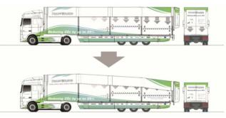
Fig. 3 Load Optimisation Combination with Double Floor Loading System and Aerodynamic Measures (adjustable roof, boat tail, side skirts)
