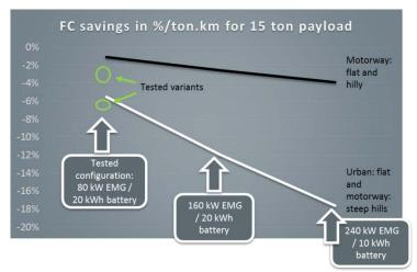
Fig. 6 Fuel saving potential of different HoD configurations based on real world testing and simulations
