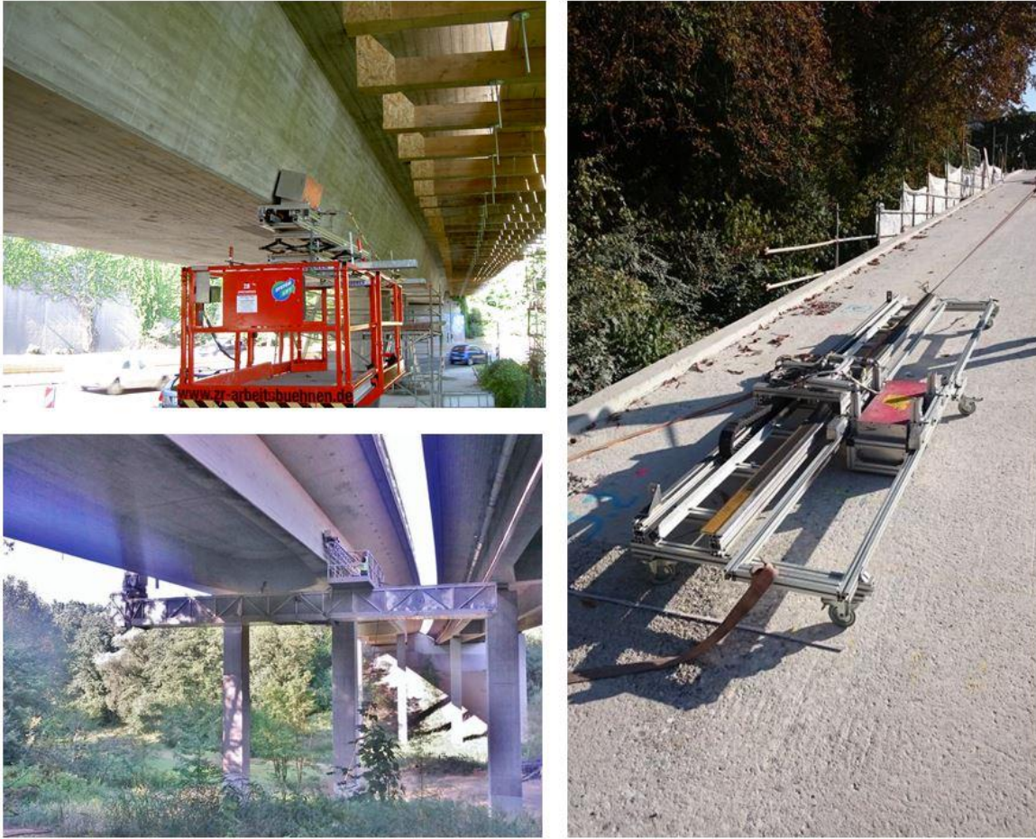
Fig 5: Top left: Bridge near Würzburg, measuring the underneath and side strands with a scissor lift. Bottom left: Bridge in northern Bavaria, measuring the underneath and side strands with an underbridge inspection unit. Right: Bridge near Karlsruhe, measuring the topmost strands with a measurement system designed and constructed at the MPA Stuttgart
