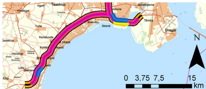
Figure 7: The M10 motorway in Denmark; the blue sections are vulnerable to flooding. (ROADAPT, 2015)
