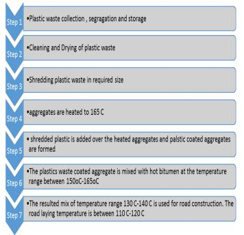
In wet process, we use waste plastic for modification of bitumen; where as in dry process, waste plastic is used for coating over aggregates.
