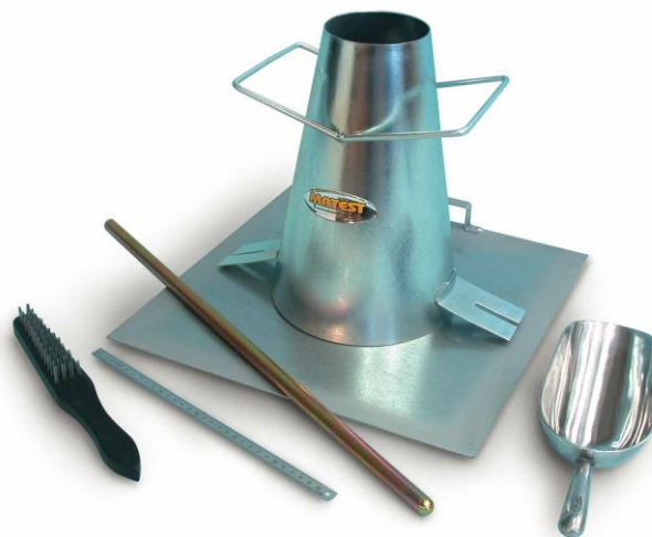
Figure1. Slump Cone Test
