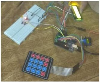
Fig1. The working of a door locks system when a wrong code is entered
