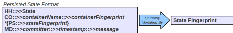
Figure 7.9: Persisted State Format for Calculating Fingerprint
