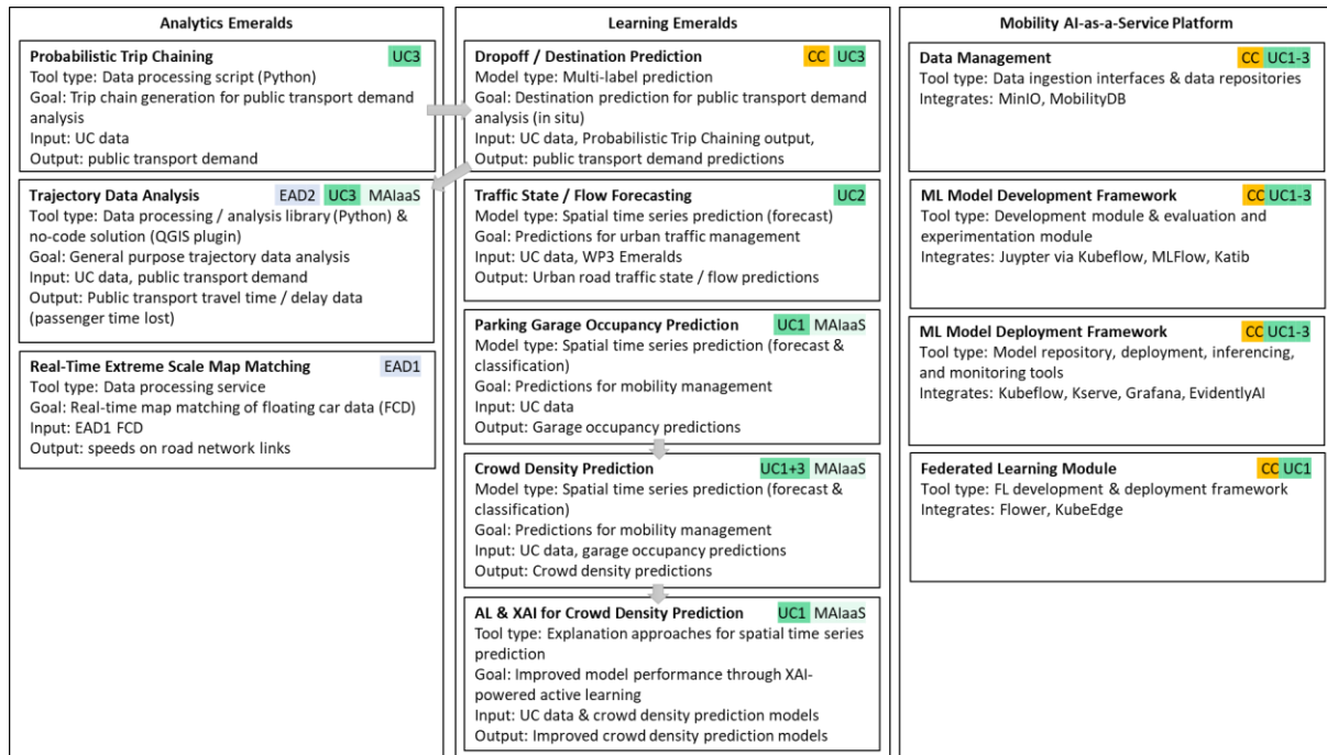
Figure 1-1: D4.1 Software components / emeralds and their role in mobility data analytics as a service
