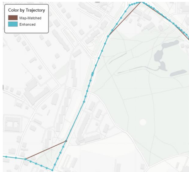
Figure 3-4 - Enhancing the map matched trajectory with the Curve Interpolation and Trajectory Refinement algorithms
