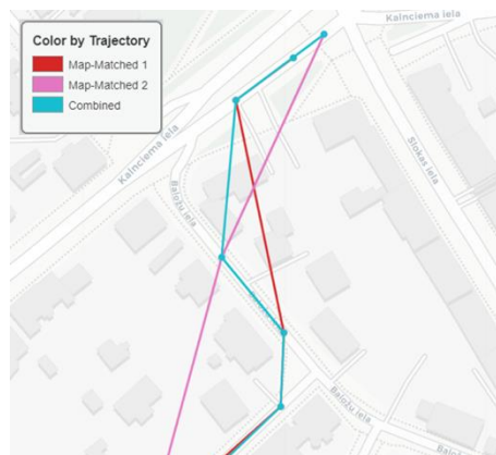
Figure 3-5 - Enhancing the Map Matched trajectory with the Trajectory Combination algorithm.
