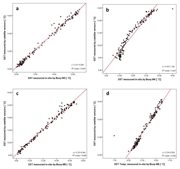
Fig. 7 a-d: Scatter plot of the satellite sensor and buoy SST data at the location of the (a) M3 buoy (51.2166 °N, 10.5500 °W), (b) M4 buoy (54.9982 °N, 09.9922 °W), (c) M5 buoy (51.6900 °N, 06.7040 °W) and (d) M6 buoy (53.0748 °N, 15.8814 °W) in the period from 01.01.2009 to 31.12.2010 at 5-day intervals [  $^{\circ}$ C].
