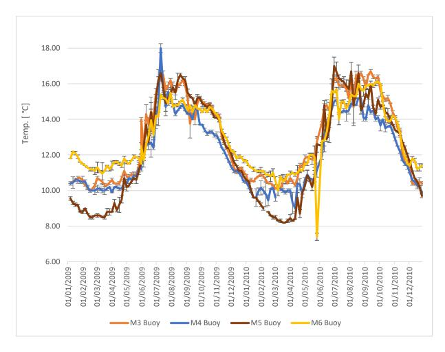
Fig. 5: Median sea surface temperature for the four Met Éireann buoys from 01.01.2009 to 31.12.2010 at 5-day intervals as measured at approximately 1 m depth [IQR as a measure of uncertainty].
