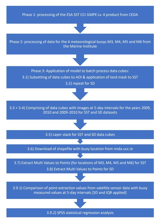
Fig. 4: Schematic of data processing steps from Phase 1: processing of the satellite data, Phase 2: processing of the buoy data to Phase 3: processing of the match-up data.
