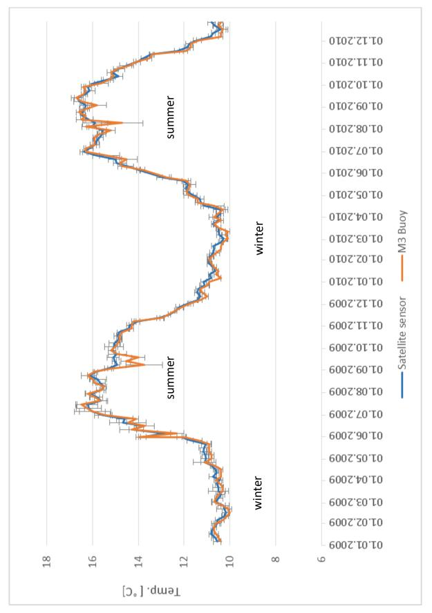
Fig. 6a: Median sea surface temperature at the location of the M3 buoy (51.2166 °N, 10.5500 °W) from 01.01.2009 to 31.12.2010 at 5-day intervals as measured by the M3 Buoy at approximately 1 m depth [IQR as a measure of uncertainty] and the satellite at 20 cm depth [SD as measure of uncertainty].
