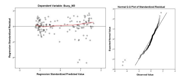
Fig. 10a: : Residual diagnostics and Q-Q-plot for the satellite sensor and buoy SST data at the location of the M3 buoy (51.2166 °N, 10.5500 °W) in the period from 01.01.2009 to 31.12.2010 at 5-day intervals.
