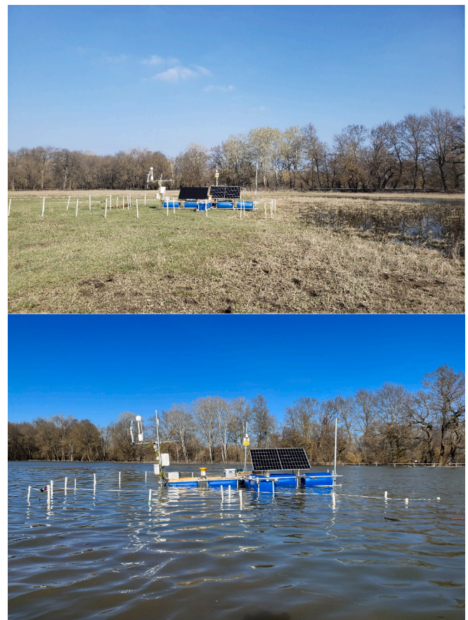
Fig. 2. EC station in the WWF - alluvial reserve at Marchegg on the grassland in March 2024 (upper), and flooded in February 2024 (lower). To solve power issues a second solar panel was added end of February 2024.
