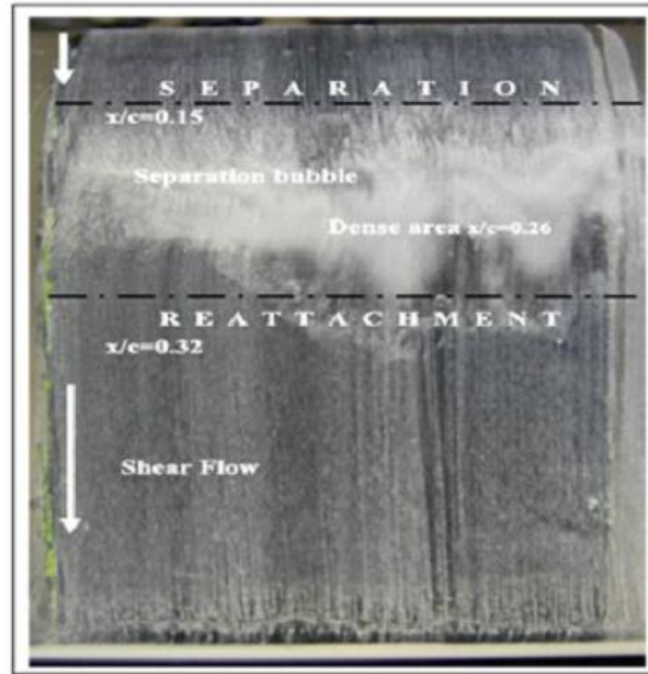
Fig. 14: Oil flow visualization over NACA 2415 airfoil at 8-degree angle of attack [72]
