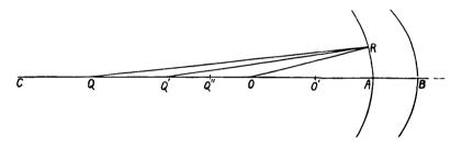
We shall suppose that the incident ray makes a small angle with the axis.
