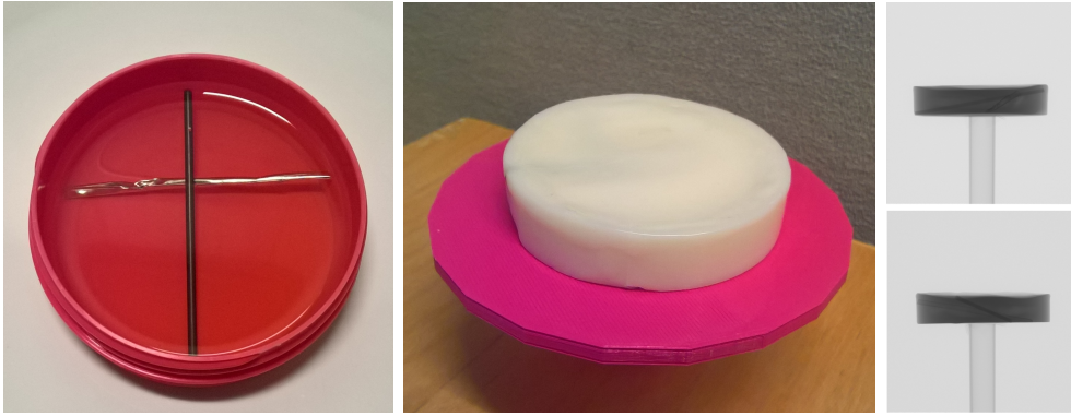
Kuva 2: Left : The phantom in the preparation phase, when the positions of the sticks were set. The darker stick is a graphite taken from a pen. The aluminum stick was made by rolling aluminum sheet, which explains its irregular shape. It is also hollow and contains air, which can be seen in the resulting reconstructions. Middle : The ready-made phantom on the sample holder, which can be attached to a computer-controlled rotator platform on the CT device, see Figure 1. Right : Two examples of the resulting 2D projection images.
