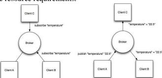
Fig 4. PUBLISH AND SUBSCRIBE MECHANISMS IN MQTT PROTOCOL
