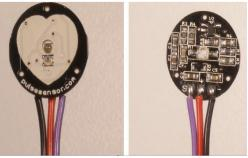
Fig 1. PULSE SENSOR
