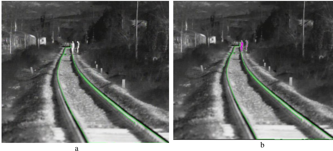
Fig. 5 (a) Thermal image of unilluminated rail crossing during night with rail tracks detected; (b) Detected object on the rail track
