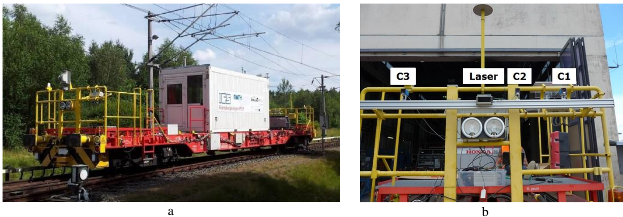
Fig. 3 (a) IFS Research Vehicle used in SMART evaluation scenario; (b) Sensors mounted on the front rail of the IFS Research Vehicle for the purpose of preliminary tests
