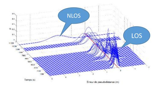
Fig 3. Pseudo-range error distribution versus time for LOS and NLOS received satellites (Viandier 2011)
