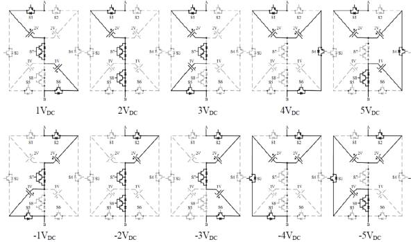
(b) Switching sequences Fig. 3 E-Type module MLI of proposed system
