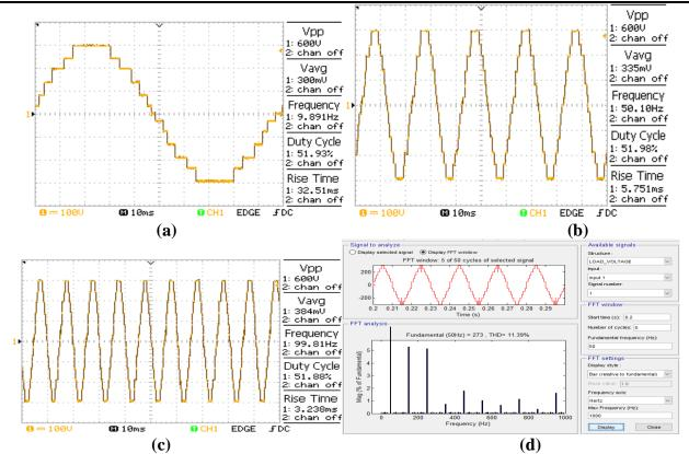
Fig.6 FFT analysis and Output voltage of proposed system
