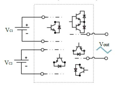
Fig.2 The basic structure of asymmetric MLI
