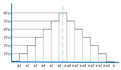
Fig.5Shows the waveform of Selective harmonic elimination modulation to find αi (Quarter wave symmetry)
