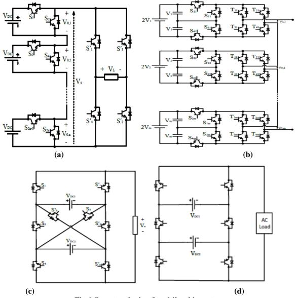
Fig.1 Sometopologies of multilevel inverter
