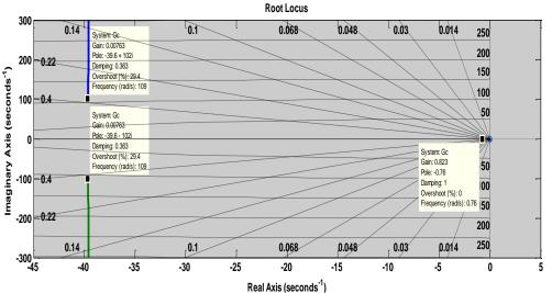
Fig 5: Root Locus of Closed-Loop System using a PID Controller.
