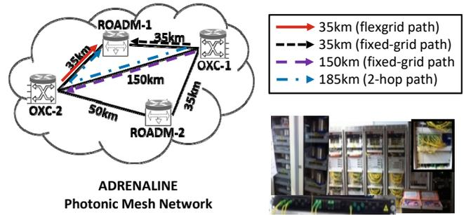
Fig. 2. ADRENALINE network paths and testbed picture.
