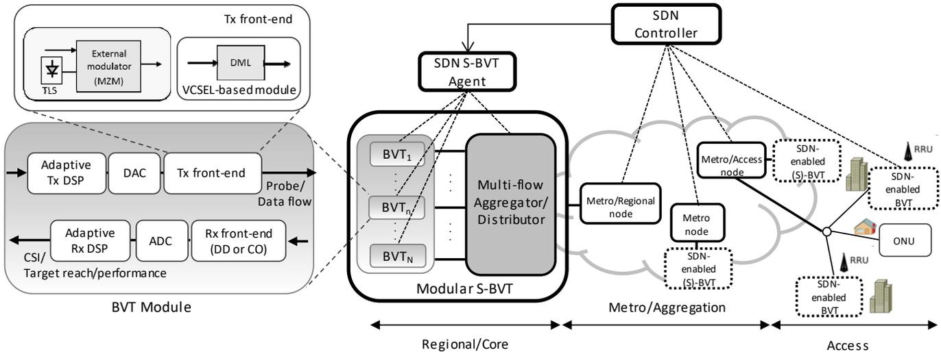
Fig. 1. Schematic architecture of an SDN-enabled modular S-BVT to be suitably sized according to the network/node needs and related scenario.
