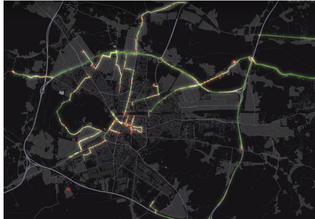
Fig. 7 Traffic density map view. Green represents light, orange medium, and red dense traffic density.
