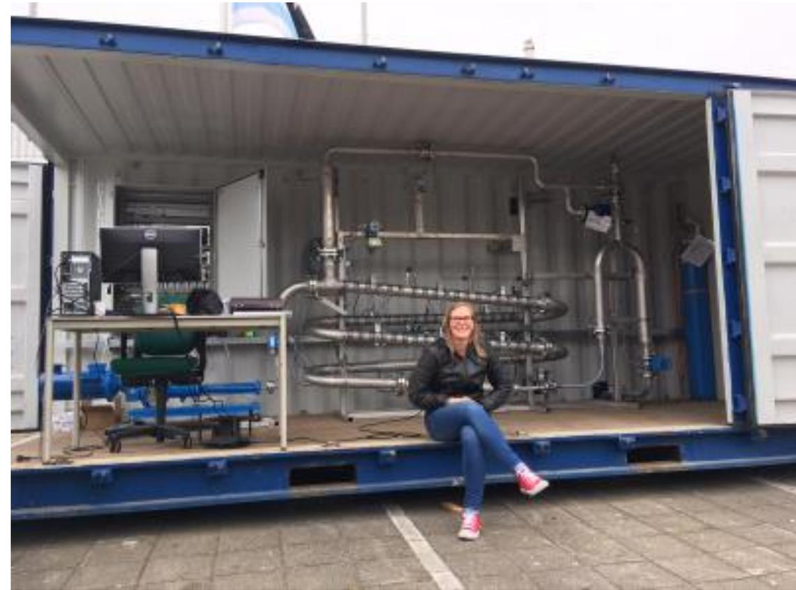
**Mobile TORWASH installation for sludge**
