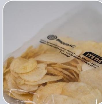
Transparent compostable / biodegradable PLA film reinforced with BNC, NL and self-cleaning antibacterial surface with nanoimprint lithography
