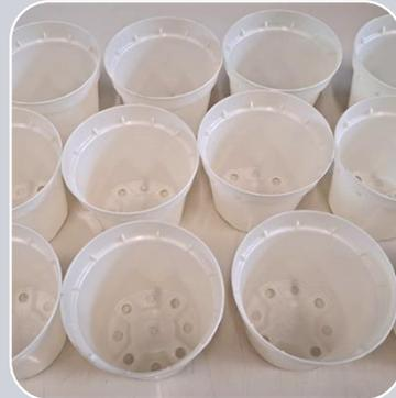
Recyclable and biodegradable bioplastics based on biopolymer (LA, SA-derived) nanocomposites with NFC, NL (1-3%) and biochar
