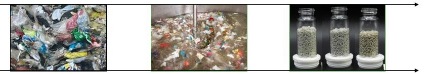
From waste plastics via sorting and mechanical recycling to granulates and products
