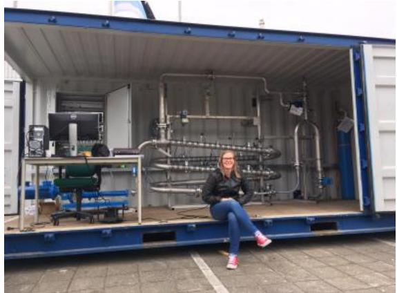
Mobile TORWASH installation for sludge
