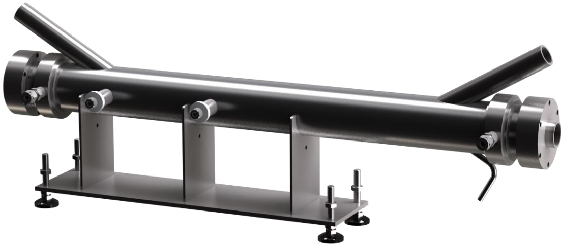
Figure 4: The prototype of the UV ionization chamber (without flow connection lines or the light source)
