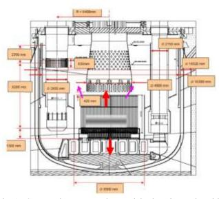
Fig. 1 ESFR Pool concept and potential relocation paths with geometrical values
