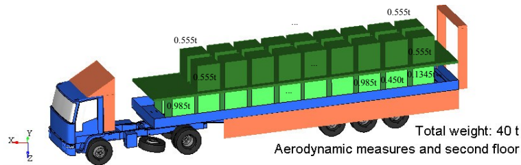
Fig. 8 Developed simulation model for truck with Load Efficiency Trailer
